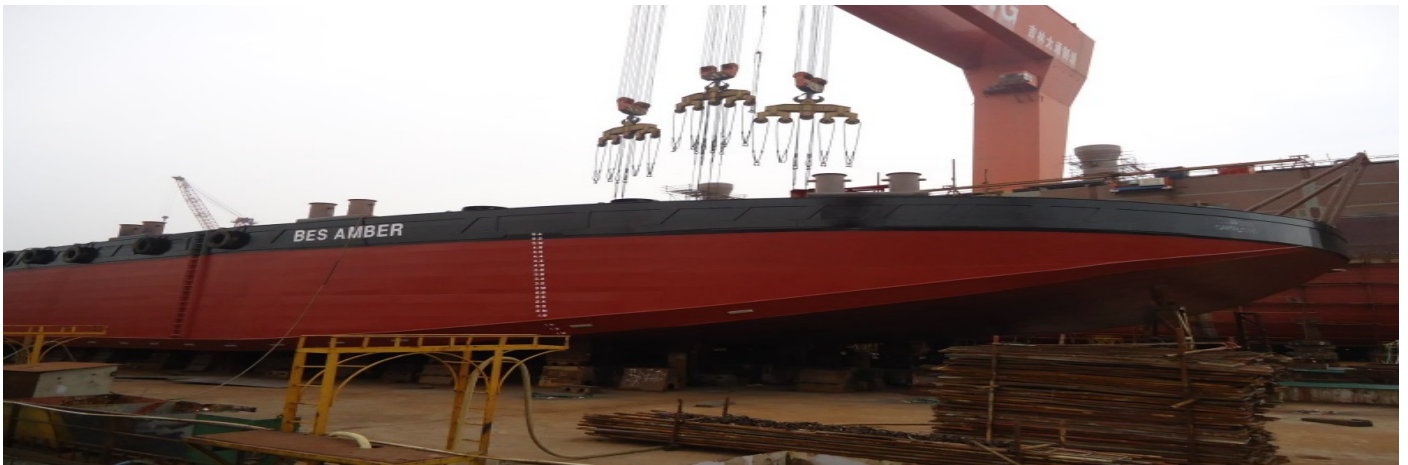
365ft x 100ft x 22ft DECK CARGO & BALLAST TANK BARGE
